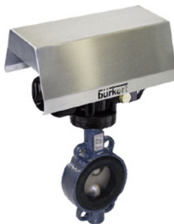
Butterfly valve with stainless steel disk and rilsan coated pneumatic actuator and 8793 positioner + process controller; with protective hood. Unit assembled for use in an ancillary process in a dairy processing plant.
